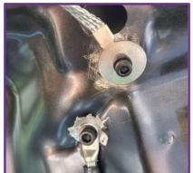
You don't need to buy an expensive tool to use rivet nuts. I saw YouTube videos describing multiple ways to install them using common wrenches, nuts and washers. (Link)
