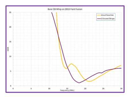
I then connected my NanoVNA and swept VSWR from 2-30 MHz. Here's the plot it generated. The SWR is not significantly different than before which leads me to think that improving the grounding between the SGC coupler and the trunk and the FT-857D and the car chassis had more of an impact than the grounding on the antenna itself.
