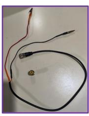
the short cable I made from an old RG-58 jumper cable. I attached 12" leads with alligator clips to one end. The leads had to be this long to reach the center terminal braid and ground braid in the trunk. Adding this cable will lower the resonant frequency measurement somewhat, so that must be factored in.
