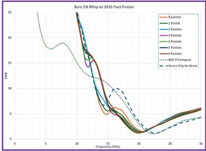
Changing wire from SGC coupler to antenna mount: To try to reduce coupling between the antenna hot lead and the trunk lid where it attaches to the antenna mount, I replaced the shielded ground strap with a simpler 8" section of 14AWG wire. This has a much smaller diameter than the RG-8 shield inside of a  $\frac{1}{2}$ " plastic gas line that I was using before.
