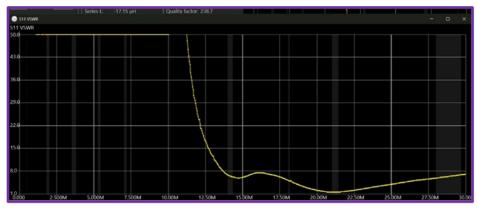
Here's the NanoVNA screen capture from the NanoV-NASaver program. It confirms that I can tune this antenna on the 20m and higher bands. Below around 12MHz, the VSWR quickly goes to infinity (set at 50:1 on this graph to make it readable). See the Excel chart on the next page of the same data – it's easier to read.
