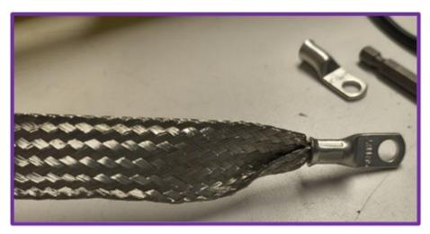
I created ground straps from 1-inch RF braid. Doing some research, I determined that 4 AWG lugs are the right size to crimp to the RF braid. I then added heat shrink tubing to protect the ground braids from weathering.
