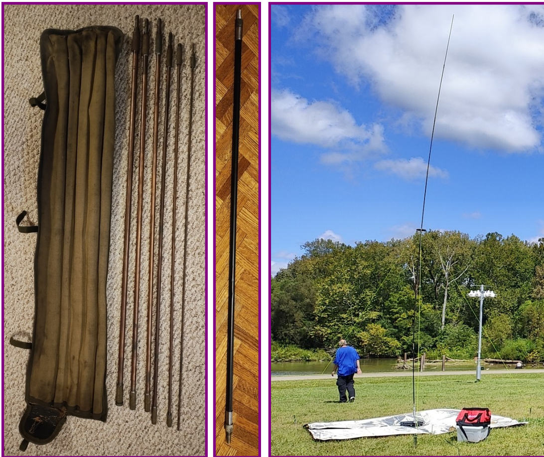
Figure 1 - BG-56A Antenna Bag with 6 Antenna Mast Sections, Dual-Threaded Mast Adapter, and Full Antenna Deployed
