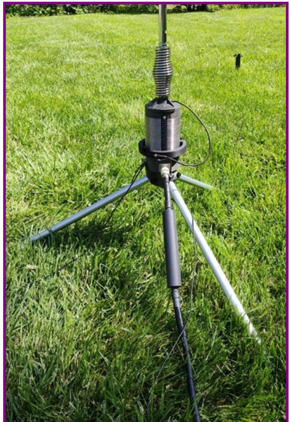
Figure 1- BKC tripod, spring, bayonet quick disconnect, radials
