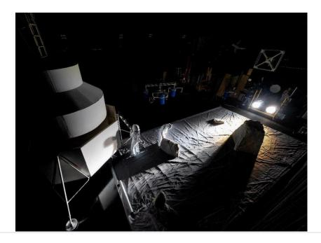
Using high-intensity lighting and low-fidelity mock-ups of a lunar lander, lunar surface, and lunar rocks, NASA engineers are simulating the Moon's environment to study and experience the extreme lighting environment at the lunar South Pole.
