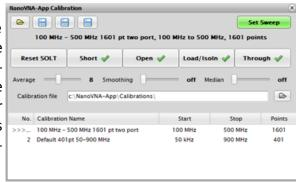
Now that the calibration is done, the fun can begin. Put NanoVNA-App in Continuous Scan mode. Connect a typical dual band handheld antenna to CHO. The graph area defaults to showing **Freq Log Mag dB S**<sub>11</sub> which is mathematically related to VSWR by the formula:
