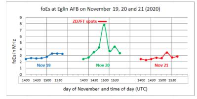
Here's that plot. Multiplying foEs by 5 gives an approximation for the MUF for a 2000 km Es path of around 40 MHz. The spike in foEs occurs only on the 20th at the time of the ZD7FT spots. It suggests that 28 MHz could have been supported on the K9LA end for a short time. Was the spike in foEs on the 20th be the enabler for my ZD7FT QSO?
