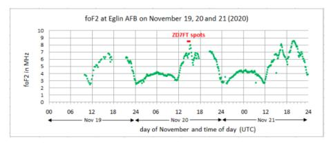
Let's now look at more detailed data from the Eglin AFB ionosonde data on the day before, the day of the ZD7FT spots and the day after. First, here's the plot for foF2 – the F2 region critical frequency. Multiplying foF2 by 3 gives an approximation for the MUF for a 3000 km F2 path. The MUF for a 3500 km path (that works out to 3 hops from ZD7FT to K9LA) would be a bit higher at about 28 MHz. The
