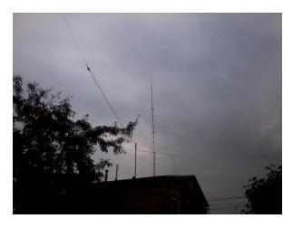
vertical dipole. It suits me: low angles of radiation, multibandwidth and a small area for its installation. I had to modify my antenna: replace the capacitor at the top with a more powerful and different nominal and play with the length of the elements.
