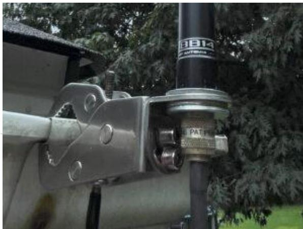
The fully-assembled antenna-and-feedline “sandwich”
