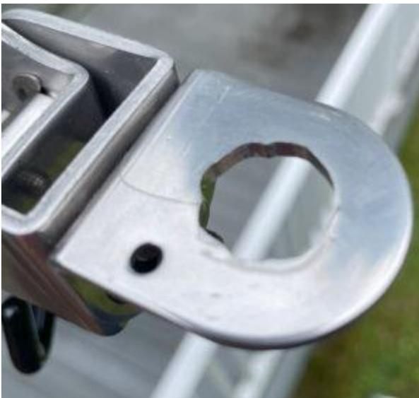
The clamp with the hold bored out to 5/8" (click to enlarge)
