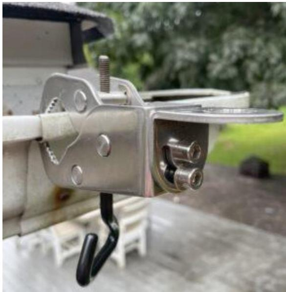
The clamp attached to the gutter.
