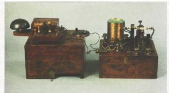
Marconi’s wireless receiver, built in 1895.
