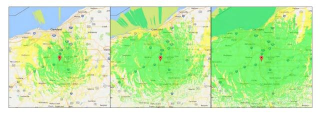
Copley TWP DMR repeater range and coverage model using a handheld radio, left, a mobile radio, center, and base station, right.
