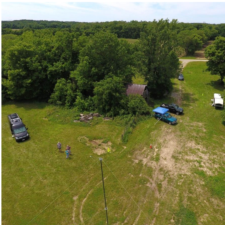
Phone operation on the left, 160-meter Windom supported by two 40' masts (second mast 265' left of the one shown) CW operation on the right, tree supported fan dipole Generator central
