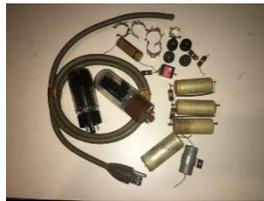
With the 75S-1 receiver completed it was time to rebuild the 516F-2 power supply unlike the 75S-1 receiver I decided to replace everything except the transformers and chokes in it. I also decide to use a circuit board in the base of it that also provided a relay to switch on and off the power so the high current spike would not go through the switch in the 32S-1 transmitter, this also
