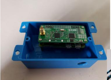
I used the hole in the side of the box that you would normally use to run your electrical wires through. This allows me the ability to run my cabling neatly
