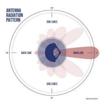
GPS satellites are not designed to assist spacecraft. They focus their radio energy on Earth where we use the signals for terrestrial navigation. So how do the MMS probes do it? The answer is "side lobes." This diagram shows a simplified but typical GPS antenna pattern:
