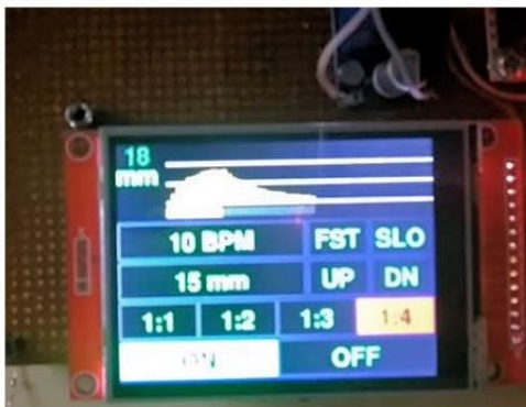
Ventilator controller interface.
