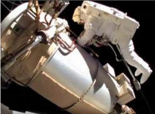
This past week, astronauts on the ISS performed troubleshooting tests on all four new feed lines installed on the *Columbus* module. One cable was earmarked for the ARISS station, while the other three are for Bartolomeo. ARISS reported over the weekend, however, that it was unable to establish communication using any of the feed line cables connected to the ARISS radio system, which was tested in APRS mode.
