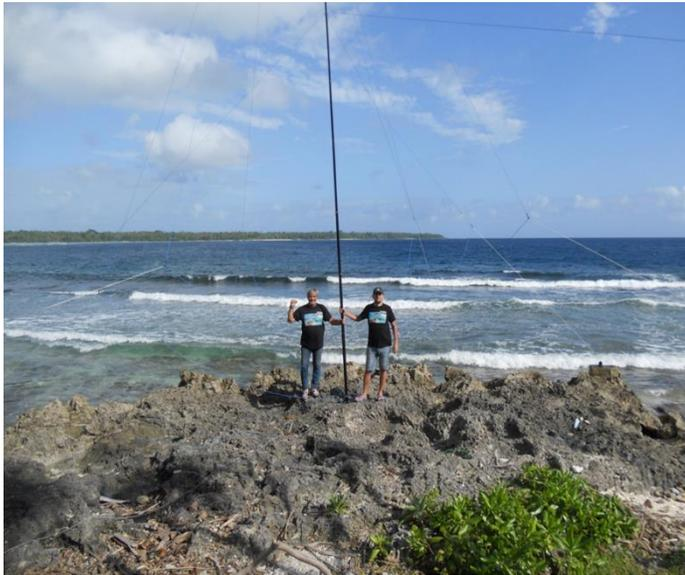
Stan. LZ1GC (L) and Lubo. OM5ZW (R) with Multiband GP antenna on made on high bands to hopefully satisfy many with ATNO's.
