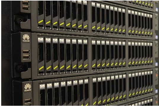
Storage server supporting RAID (Wikipedia)
