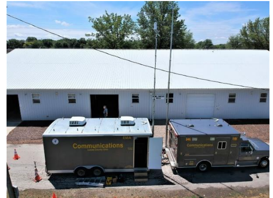
An overhead view of the Incident Command Post. The truck can be separated from the trailer to deploy to another area during widespread emergencies and has near identical radio capabilities as the trailer. (Photo Credit: Brad Ruhberg WB8RG)
