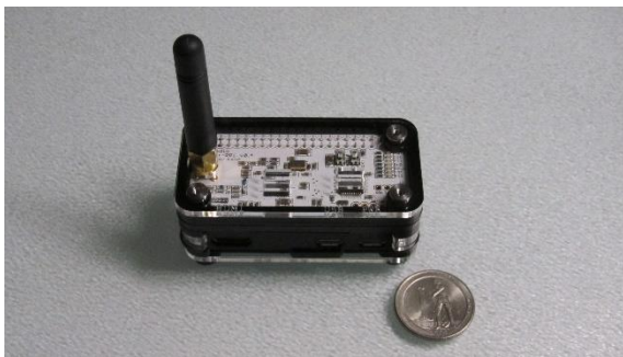
Pi Zero W with ZUMSpot GPIO HAT board, compared to a quarter
