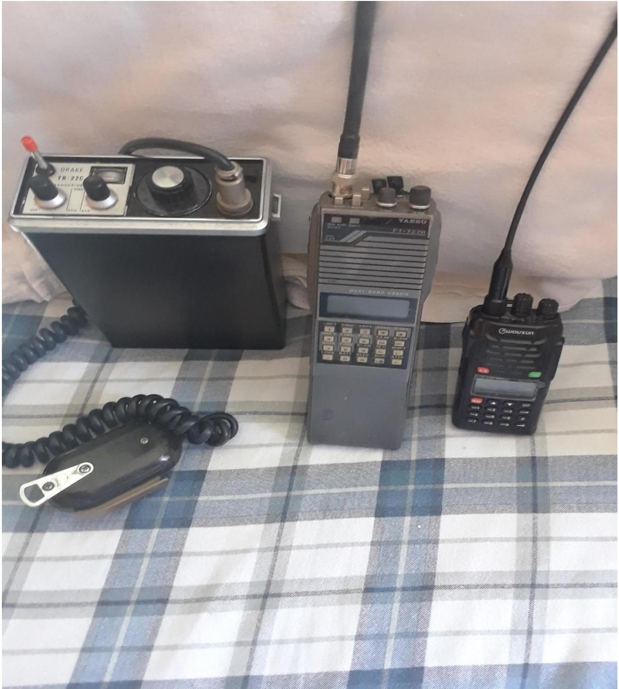
Here is a comparison of the change in the size and operation of 2 meter “hand held” radios. The one on the left is a Drake 12 channel TR-22 crystal controlled radio. The one in the middle is a Yaesu FT-727R programmable 2 meter 440 radio. Neither radio had CTCSS capabilities. The one on the right is a Wouxun KG-UVD1P programmable 2 meter 440 radio with both touch tone and programmable CTCSS tones.
