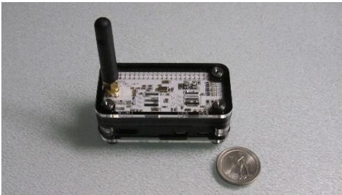
ZUMSpot on Raspberry Pi Zero compared to a quarter
