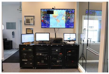
W1AW digital equipment Rack 1: APRS/D-STAR/HF MARS. Rack 2: Demo. Rack 3: Echolink & Winlink. Rack 4: IRLP
