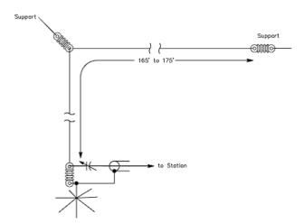
So, I thought about an inverted L antenna. This is a generic, baseline design for any inverted L antenna:
