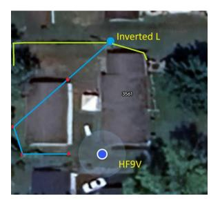
The light blue dot is the feedpoint and my aluminum mast (26' to the horizontal wire). The blue line is the wire. The red dots are supports for the wire, in order from the mast: 31', 27', 15' and 12'. The green lines are counterpoise wires. 3 are on the top of my cyclone fence at 4', left (66', 33' and 16"), and 2 are next to my attached garage, also at 4". You can see the position of my HF9V, darker blue dot.
