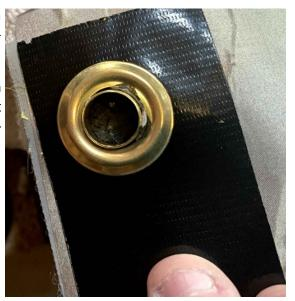
To secure the pieces together permanently, tap on the extended male portion to force the edges out and down around the female brass. I set this up using a small anvil as the base.
