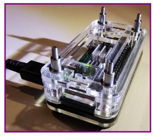
Here's the case partially built up. I assembled the bottom and installed the Pi-Zero 2W and stopped assembly at the point where the N5BOC modem would be installed. Having not yet received the modem, I installed WPSD and configured it as much as I could with no modem and checked the heat dissipation. Heat was not an issue, the CPU never reported a temperature above 51° C.
