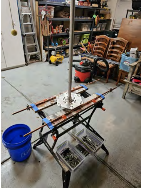
Figure 7: Mast plate and feed point in place—ready for spreaders
