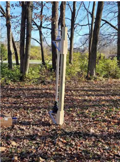
Figure 5: 4x4, rotor, and thrust bearing on “tower” portion. Looks crooked, doesn’t it?
