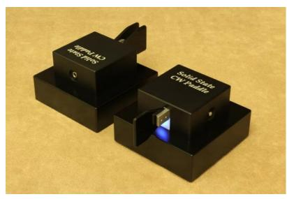
**9A5N**: Thanks to my friends, top class telegraphists, Bero 9A5KR and Daki 9A2WJ (both SK) and endless discussions about the shortcomings of mechanical CW keys and paddles, I invented the Solid-State CW Paddle 10 years ago. As the paddle has no moving parts and bearings, no contacts and no springs / magnets, it is completely immune to dust, oxidation and temperature changes, requires no maintenance and keying with it is completely silent. Only the
