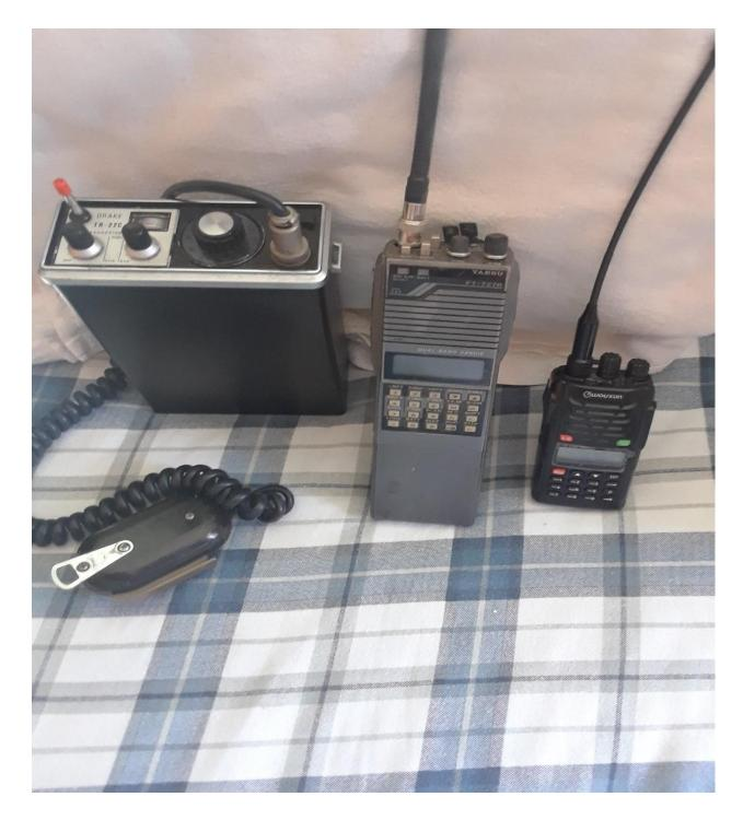
Here is a comparison of the change in the size and operation of 2 meter "hand held" radios. The one on the left is a Drake 12 channel TR-22 crystal controlled radio. The one in the middle is a Yaesu FT-727R programmable 2 meter 440 radio. Neither radio had CTCSS capabilities. The on the right is a Wouxun KG-UVD1P programmable 2 meter 440 radio with both touch tone and programmable CTCSS tones.
