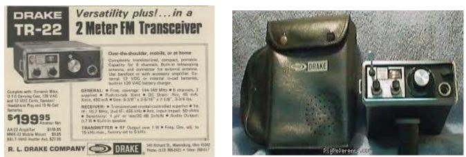
1971 Drake TR-22 Crystal controlled 2 meter hand held radio
