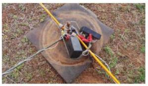
This shows the feedpoint for three Beverages at a single point, each one selected using a remote controlled relay.
