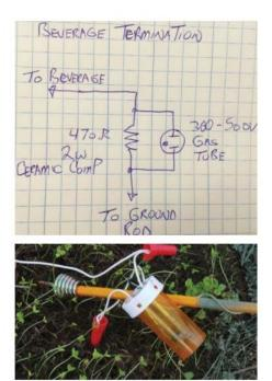
Above is the schematic for the termination end of the beverage. The picture shows one actually installed. Another "pill bottle" is used here. Note the wire nuts making the connections.
