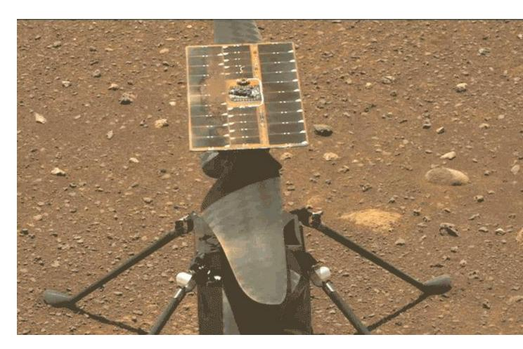
Mastcam-Z Captures Ingenuity's Blades Spinning: The Ingenuity Mars Helicopter's carbon fiber blades can be seen in this video taken by the Mastcam-Z instrument aboard NASA's Perseverance Mars rover on April 8, 2021, the 48th Martian day, or sol, of the mission. They are performing a wiggle test before the actual spin-up to ensure they were working properly. Credits: NASA/JPL-Caltech/ASU. Download image >
