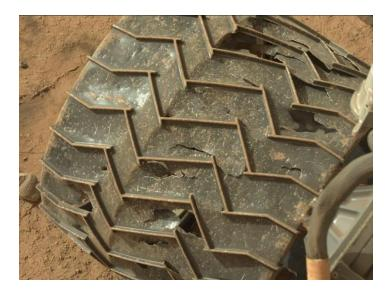
This image of wear and tear damage sustained by the <u>wheels</u> of NASA's Curiosity Rover was taken on Feb. 7, 2022, nearly a decade after the craft first began to explore the Martian surface.
