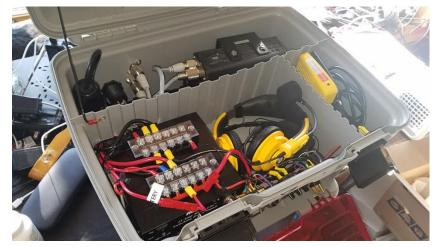
it has MFJ Mighty Lite 25 amp power supply build in, and Power Pole connection to connect to a battery.
