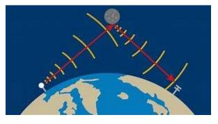
For terrestrial use the FT8 decoder searches over the range -2.5 to +2.4s for clock offset DT between transmitting and receiving stations. When "Decode after EME delay" is checked on the WSJT-X "Settings" screen, the accessible DT range becomes -0.5 to +4.4 s. Just right for EME.
