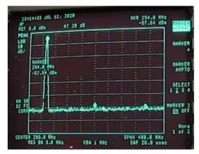
Alinco DJ-F1 on a Spectrum Analyzer. Left most spike is the fundamental frequency. The diamond marker in about the middle of the noise floor is the first spurious emission. This emission is -57 dBm (upper right) form the fundamental. This radio is compliant with Part 97 as it is beyond -40. (The Radio Mechanic YouTube
