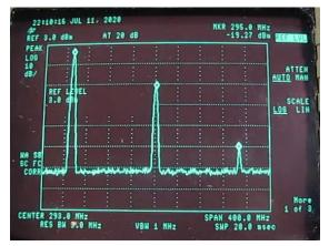
Baofeng UV-5RX3 on a Spectrum Analyzer. Left most spike is the fundamental frequency. Next spike to the right of the fundamental is the first spurious emission. This emission is only -19 dBm (upper right) from the fundamental. These emissions are nowhere near -40 or Part 97 compliant. (The Radio Mechanic YouTube video)
