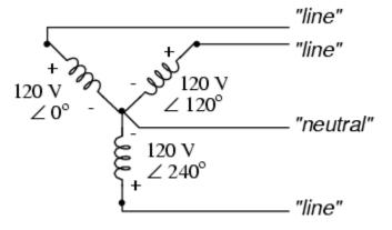
The neutral is NOT ground (unless it is grounded of course). Let's use 208Vac 3-phase Y-connected as an example. Also, take a glance at the fancy pic that I found on Google.
