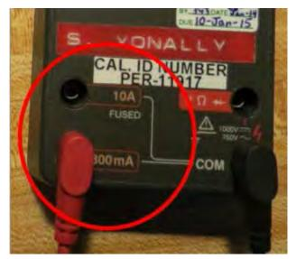
I will tell you that on this particular meter it really doesn't change the reading, as all of you pointed out to me in the first boo-boo above. But, for safety sakes, it is important that you have the connections to the meter correct as well. This is so you are operating everything in a fused circuit, and not just hanging it out there where you could potentially burn up the meter, or worse, YOU.
