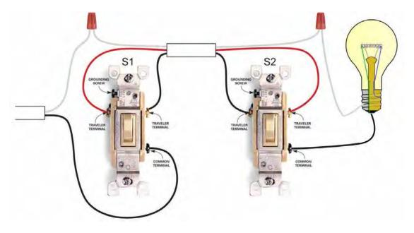
control a light at 2 different locations. I do want to mention that these switches are designed to be operated this way, so you can't use just any switch to do this. If you look close at the diagram, you'll see that 3-way switches have an additional terminal on them. This is for the traveler wire. It's what makes this all possible.
