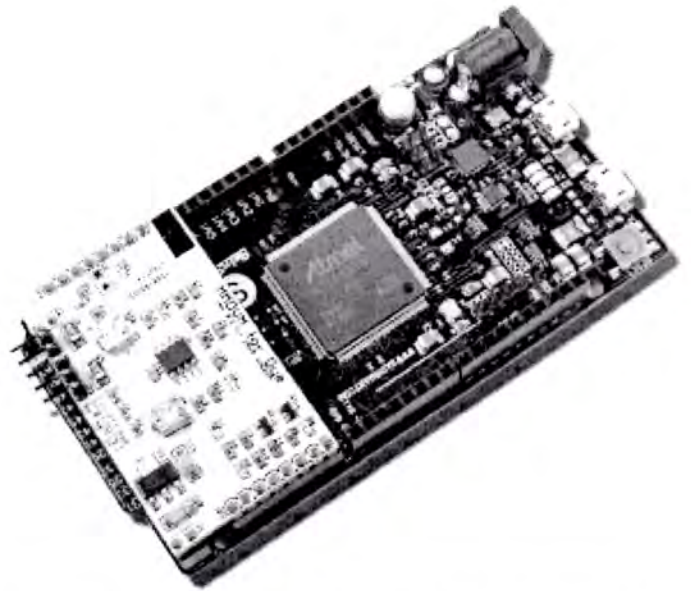
Left: The TYT MD-390 is the latest in a popular line of single-band portables aimed squarely at the amateur radio market. (Courtesy of Universal-Radio) Right: The MMDVM mounts on to an Arduino SBC – then connects through a Raspberry Pi SBC to complete a homebrew DMR repeater with networking capabilities. (Courtesy of gb7dd.co.uk)
