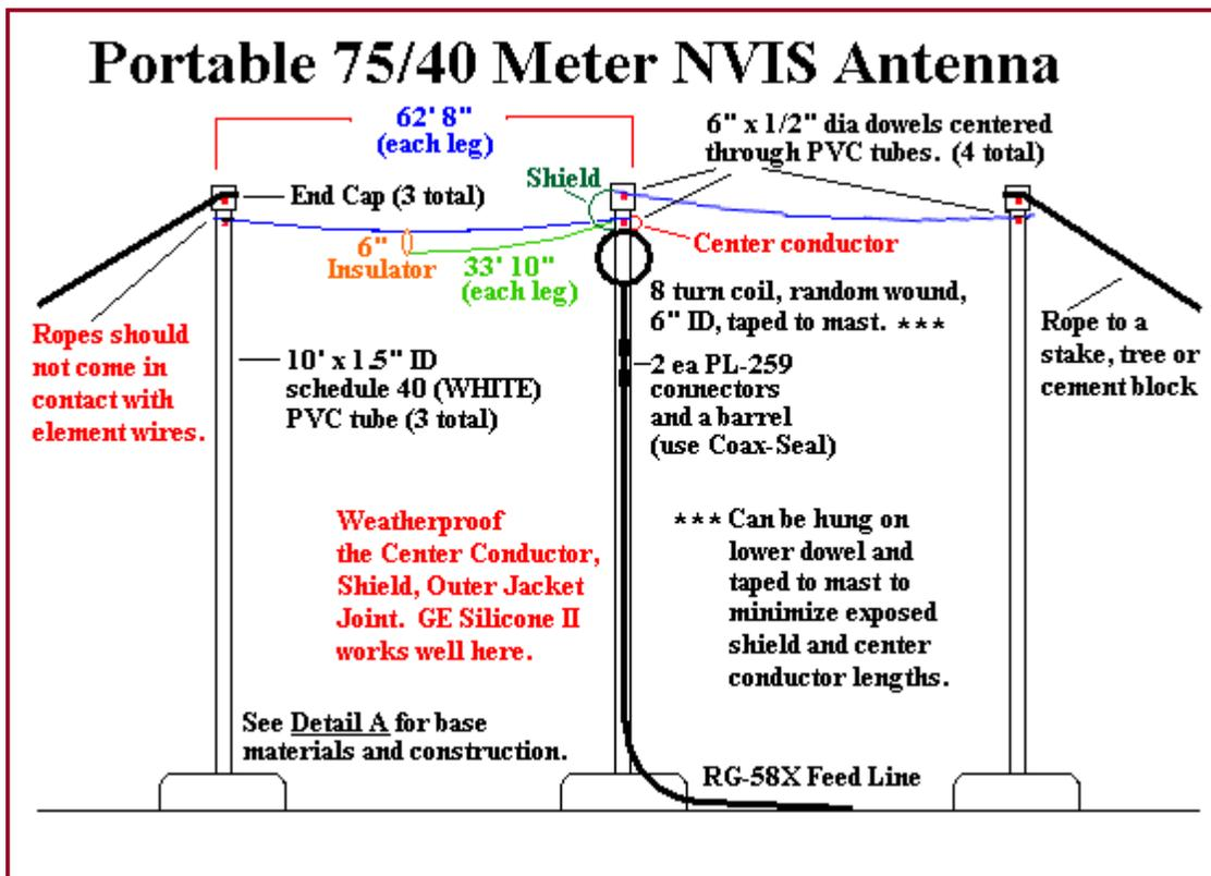
5. Repeat for the element connected to the shield braid, hanging it on the top dowel at the center mast.
